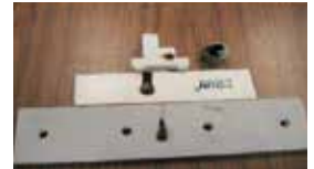
Grow-wire test at 960 Degree Celsius.
